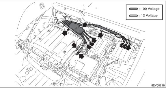
(2) Remove the nut and disconnect the power cable positive terminal from the 12 volt auxiliary battery.
