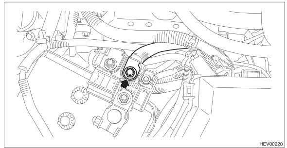
(3) Release the power cable clamp and the power cable clip.
