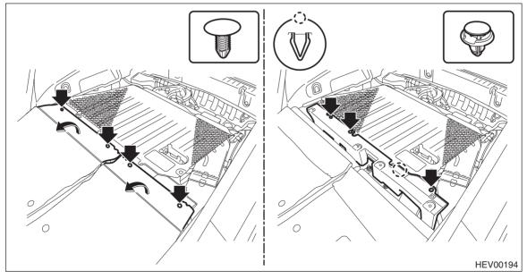
5) Remove the TORX<sup>®</sup> bolts, release the clips, and then remove the battery cover.
