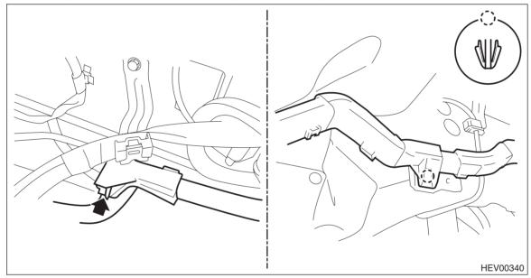
(4) Remove the bolt, then remove the power connect cover and the gasket.
