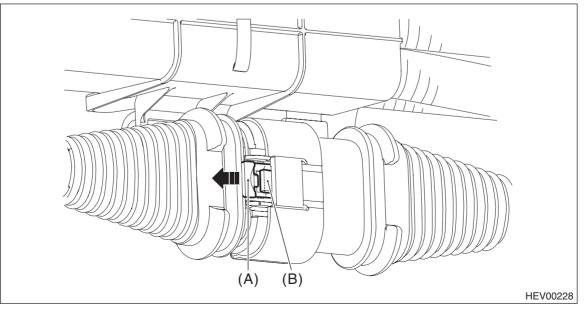
(7) Remove the bolts and nuts, release the clips and claws, and disconnect the power cable from the vehicle.
